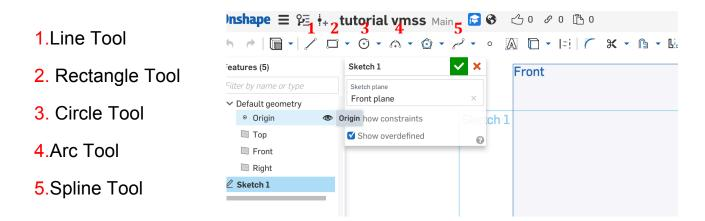
7. The end result of using the tools should be a "closed shape." When the shape is "closed" the inside will be light gray in color…
