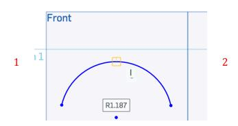
8. When the shape is "closed" the inside will be light gray in color... You can now **EXTRUDE** the shape into a 3D object.
