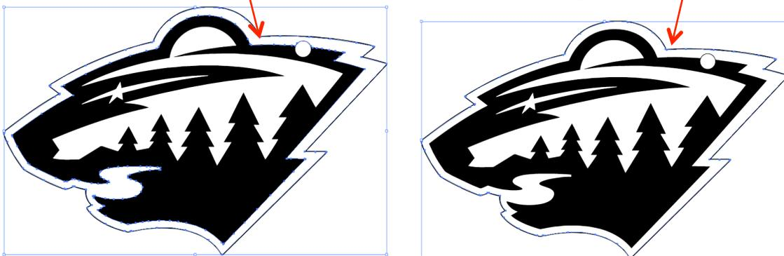
*NOW you can set the outside line's weight. The line weight is how the laser knows what lines to cut.*
